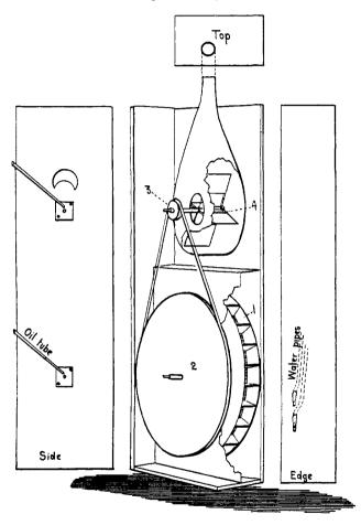
of the wheel. The larger pulley-wheel has a diameter of 10 inches, is of a good quality of white pine and was soaked for three hours in melted paraffin to prevent warping. It has a groove  $\frac{3}{6}$  of an inch for the belt. These wheels are mounted on a  $\frac{3}{6}$  inch shaft, turned down at each extremity to  $\frac{1}{6}$  inch bearing. The smaller pulley-wheel is of wood  $\frac{3}{4}$  of an inch in diameter, with flanges
